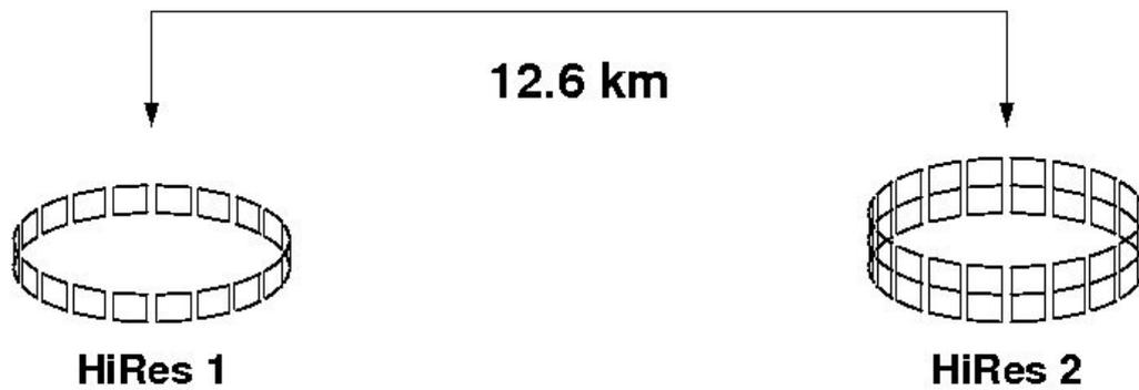
The HiRes fluorescent detector in Utah consisted of two telescopes with slightly different field of view. One of them looks at elevations of 3 to 17 degrees and the other one from 3 to 31 degrees. They can also work in coincidence.
